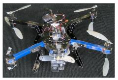
Replaced props, standoffs, bolts, antennas.
