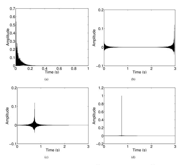
Fig. 5: Inversion process. (a), simulated impulse response  $\hat{g}(t)$ ; (b), noncausal inverse filter h(t) using regularized inversion; (c), shifted and truncated inverse filter  $\hat{h}(t)$ ; and (d), dereverberated output  $\hat{x}(t)$  ( $x(t) = \delta(t)$ ).
