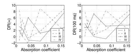
Fig. 15: Dereverberation ratios with respect to absorption coefficient  $\bar{a}$ .
