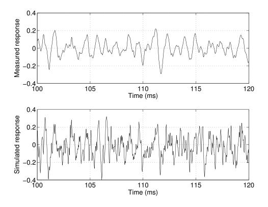
Fig. 10: Measured and simulated impulse responses after 100 ms.
