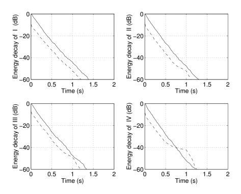
Fig. 18: Integrated energy decay curves for scalar inversion. Solid line is measured response; dashed line is dereverberated response.
