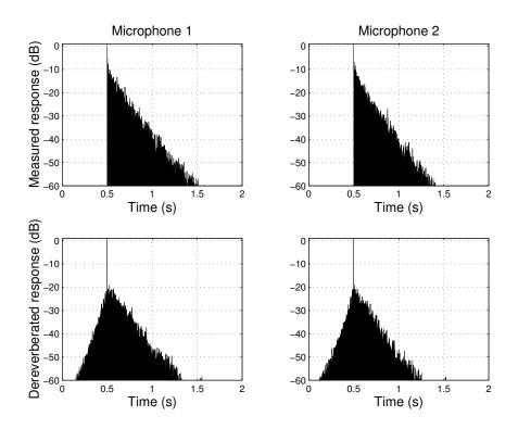
Fig. 20: Decibel plots of measured and dereverberated impulse responses ( $2 \times 2$  matrix inversion). An exponential window with time constant  $\tau = 0.06$  s is applied to the simulated impulse response  $\hat{g}(t)$ .
