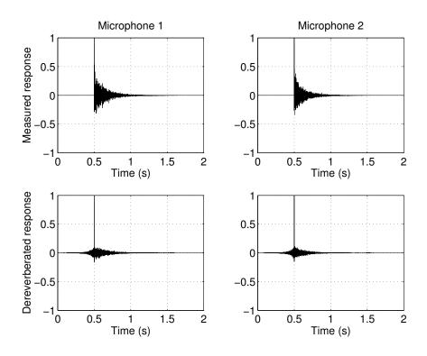
Fig. 19: Linear plots of measured and dereverberated impulse responses (2  $\times$  2 matrix inversion). An exponential window with time constant  $\tau=0.06$  s is applied to the simulated impulse response  $\hat{g}(t)$ .
