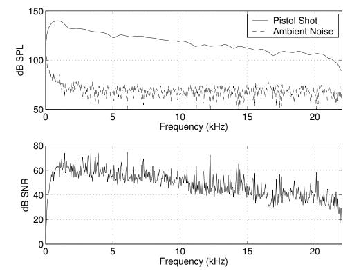
Fig. 1: Magnitude responses of starter pistol and ambient noise.
