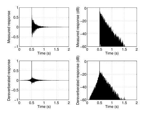
Fig. 17: Measured and dereverberated impulse responses (scalar inversion; impulse response number III). An exponential window with time constant  $\tau = 0.06$  s is applied to the simulated impulse response  $\hat{g}(t)$ .
