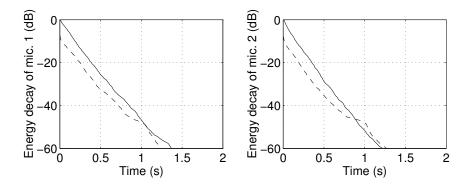
Fig. 21: Integrated energy decay curves for  $2 \times 2$  matrix inversion. Solid line is measured response; dashed line is dereverberated response.
