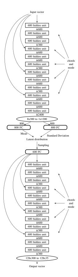
**Figure 3**: Network architecture. Rectangles are bidirectional recurrent neural network cells. Ellipses are strided time-convolution cells. Rounded rectangles are fully connected (FC) layers. Numbered arrows indicate a connection's dimension.
