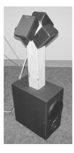
Figure 2. Quasi-spherical loudspeaker configuration for the eviolin.
